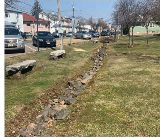
An existing rock swale can be converted to a bioswale to aid in infiltration of the stormwater runoff entering it. Additionally, the parking spaces to the west of the park can be converted to pervious pavement to capture, treat, and infiltrate the stormwater runoff from the parking lot. A preliminary soil assessment suggests that more soil testing would be required before determining the soil's suitability for green infrastructure.
